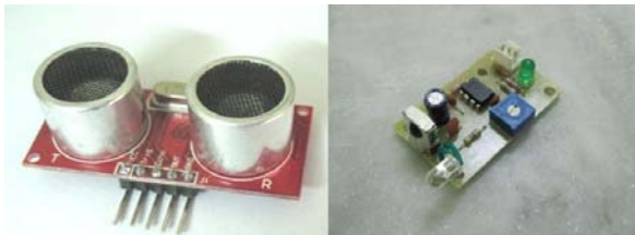
Fig. 3 Ultrasonic Sensor and Infrared Sensor
